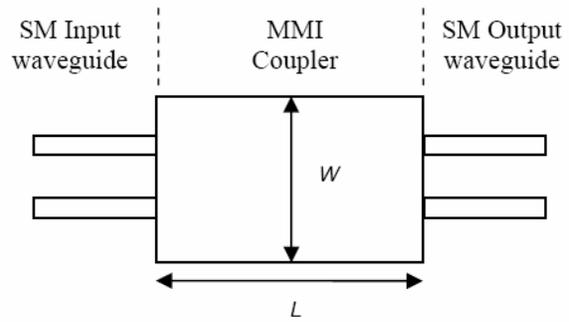
Fig. 2. Layout of the MMI cross coupler
